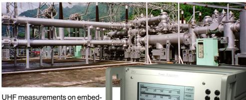
ded or external sensors are possible with the use of the RPA6C, a logarithmic preamplifier, which covers 300MHz-2GHz. As with the other preamplifiers, the AlAcompact automatically detects the RPA6C and changes into the logarith-
