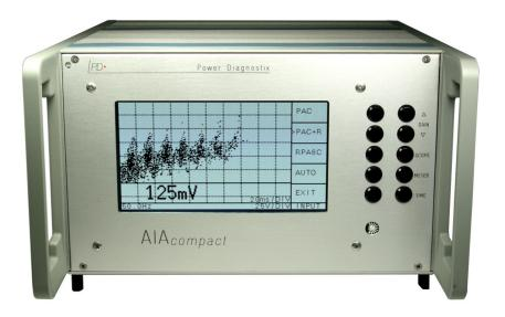
The AlAcompact is a portable unit for in-service acoustic partial discharge measurements on gas-insulated switchgear (GIS), transformers, and cable accessories. The instrument adapts to a variety of piezo-electric acoustic sensors and is supplied with a versatile sensor fixture. Additionally, the AlAcompact allows partial discharge measurements on embedded or external UHF sensors.
