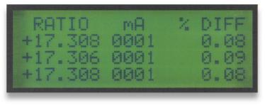
The ATRT-03B can also calculate the turns-ratio percentage error if the transformer's nameplate voltages are provided. The baseline turns-ratio is calculated using the nameplate voltages, and the test results are compared to the baseline turns-ratio. The percentage error is then calculated from the difference between the baseline and test turns-ratios.
